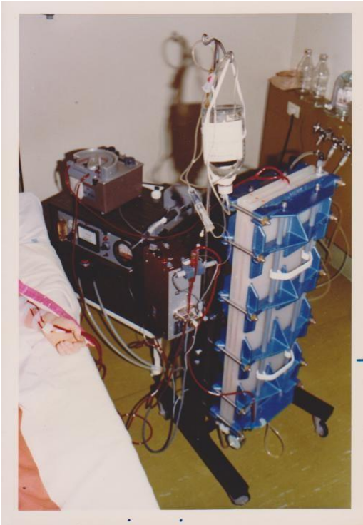
Kiil dialyser tipped ready for washback
